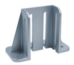
FATH foot console, silver, 8 holes, 40 x 80mm, die-cast aluminum, slot size 8. For use with all 80mm T-slotted rails. Manufacturer part number: 098G4080L85168A.
