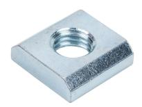
FATH slide-in nut, silver, M10-1.5, zinc plated steel, slot size 10. Package of 10. For use with all 45mm and 90mm profile T-slotted rails. Manufacturer part number: 096ST45M10.
