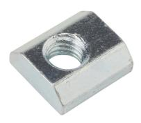
FATH slide-in nut, silver, M8-1.25, zinc plated steel, slot size 8. Package of 10. For use with all 1.5in, 3in, 40mm and 80mm profile T-slotted rails. Manufacturer part number: 096ST15M8.
