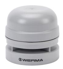
WERMA EvoSIGNAL Midi series audible signal horn, 110 dB at 1m, 3.3 kHz tone frequency, (10) selectable tone(s), 115-230 VAC, modular mount, ABS/polycarbonate housing, gray, IP66. Requires mounting adapter.
