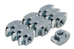
FATH hammer nut, silver, M4-0.7, zinc plated steel, slot size 10. Package of 10. For use with all 45mm and 90mm profile T-slotted rails. Manufacturer part number: 096H10430.
