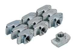
FATH hammer nut, silver, M5-0.8, zinc plated steel, slot size 8. Package of 10. For use with all 40mm and 80mm profile T-slotted rails. Manufacturer part number: 096H08530.
