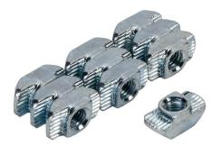
FATH hammer nut, silver, M5-0.8, zinc plated steel, slot size 8. Package of 10. For use with all 30mm and 60mm profile T-slotted rails. Manufacturer part number: 096H08515.
