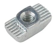
FATH hammer nut, silver, 8-32 UNF, zinc plated steel, slot size 8. Package of 10. For use with all 1.5in and 3in profile T-slotted rails. Manufacturer part number: 096H088-3215.
