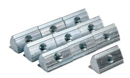
FATH roll-in nut, silver, M5-0.8, zinc plated steel, slot size 8. Package of 10. For use with all 40mm and 80mm profile T-slotted rails. Manufacturer part number: 096025F.
