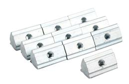
FATH roll-in nut, silver, M4-0.7, zinc plated steel, slot size 8. Package of 10. For use with all 40mm and 80mm profile T-slotted rails. Manufacturer part number: 096024F.
