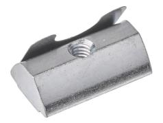
FATH roll-in nut, silver, 8-32 UNF, zinc plated steel, slot size 8. Package of 10. For use with all 1.5in and 3in profile T-slotted rails. Manufacturer part number: 09602U8-32F.
