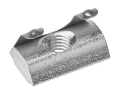
FATH roll-in nut, silver, 10-32 UNF, zinc plated steel, slot size 6. Package of 10. For use with all 1in and 2in profile T-slotted rails. Manufacturer part number: 096541U10-32F.
