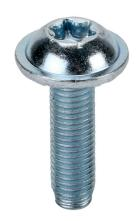
FATH T-40 Torx flange head self-tapping screw, silver, 7 x 25mm, zinc plated steel, slot size 8. Package of 10. For use with all 1.5in, 3in, 40mm and 80mm profile T-slotted rails. Manufacturer part number: 093S0725T.
