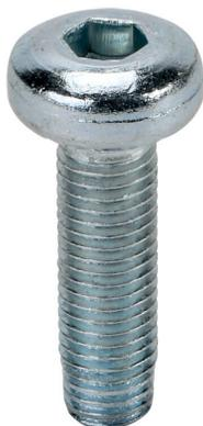
FATH button head socket cap self-tapping screw, silver, S7 x 25mm, zinc plated steel, slot size 8. Package of 10. For use with all 1.5in, 3in, 40mm and 80mm profile T-slotted rails. Manufacturer part number: 093SF0725.
