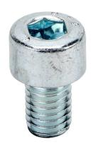
FATH socket head cap screw, silver, M8-1.25 x 12mm, zinc plated steel, slot size 8/10. Package of 10. For use with all 1.5in, 3in, 30mm, 40mm, 45mm, 60mm, 80mm and 90mm profile T-slotted rails. Manufacturer part number: 4DIN912M0812M.
