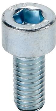
FATH socket head cap screw, silver, M6-1.0 x 14mm, zinc plated steel, slot size 6/8/10. Package of 10. For use with all T-slotted rails. Manufacturer part number: 4DIN912M0614M.
