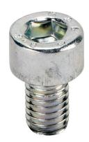
FATH socket head cap screw, silver, M6-1.0 x 10mm, zinc plated steel, slot size 6/8/10. Package of 10. For use with all T-slotted rails. Manufacturer part number: 4DIN912M0610M.
