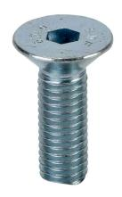
FATH flat head socket cap screw, silver, M8-1.25 x 25mm, zinc plated steel, slot size 8/10. Package of 10. For use with all 1.5in, 3in, 30mm, 40mm, 45mm, 60mm, 80mm and 90mm profile T-slotted rails. Manufacturer part number: 4DIN7991M0820M.
