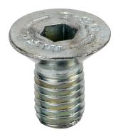
FATH flat head socket cap screw, silver, M8-1.25 x 16mm, zinc plated steel, slot size 8/10. Package of 10. For use with all 1.5in, 3in, 30mm, 40mm, 45mm, 60mm, 80mm and 90mm profile T-slotted rails. Manufacturer part number: 4DIN7991M0816M.
