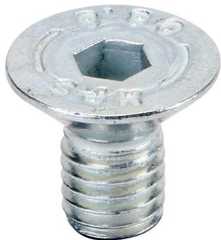
FATH flat head socket cap screw, silver, M8-1.25 x 14mm, zinc plated steel, slot size 8/10. Package of 10. For use with all 1.5in, 3in, 30mm, 40mm, 45mm, 60mm, 80mm and 90mm profile T-slotted rails. Manufacturer part number: 4DIN7991M0814M.
