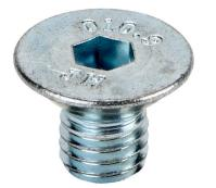
FATH flat head socket cap screw, silver, M8-1.25 x 12mm, zinc plated steel, slot size 8/10. Package of 10. For use with all 1.5in, 3in, 30mm, 40mm, 45mm, 60mm, 80mm and 90mm profile T-slotted rails. Manufacturer part number: 4DIN7991M0812M.
