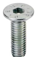
FATH flat head socket cap screw, silver, M6-1.0 x 20mm, zinc plated steel, slot size 6/8/10. Package of 10. For use with all T-slotted rails. Manufacturer part number: 4DIN7991M0620M.
