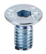
FATH flat head socket cap screw, silver, M6-1.0 x 12mm, zinc plated steel, slot size 6/8/10. Package of 10. For use with all T-slotted rails. Manufacturer part number: 4DIN7991M0612M.
