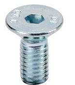
FATH flat head socket cap screw, silver, M5-0.8 x 12mm, zinc plated steel, slot size 6/8/10. Package of 10. For use with all T-slotted rails. Manufacturer part number: 4DIN7991M0512M.
