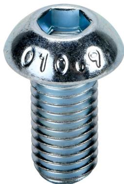
FATH button head socket cap screw, silver, M12-1.75 x 25mm, zinc plated steel, slot size 10. Package of 10. For use with all 45mm and 90mm profile T-slotted rails. Manufacturer part number: 4ISO7380M1225M.
