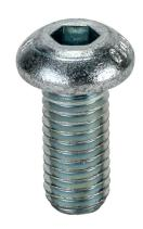
FATH button head socket cap screw, silver, M8-1.25 x 18mm, zinc plated steel, slot size 8/10. Package of 10. For use with all 1.5in, 3in, 30mm, 40mm, 45mm, 60mm, 80mm and 90mm profile T-slotted rails. Manufacturer part number: 4ISO7380M0818M.
