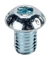
FATH button head socket cap screw, silver, M8-1.25 x 12mm, zinc plated steel, slot size 8/10. Package of 10. For use with all 1.5in, 3in, 30mm, 40mm, 45mm, 60mm, 80mm and 90mm profile T-slotted rails. Manufacturer part number: 4ISO7380M0812M.
