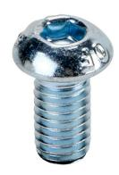
FATH button head socket cap screw, silver, M6-1.0 x 12mm, zinc plated steel, slot size 6/8/10. Package of 10. For use with all T-slotted rails. Manufacturer part number: 4ISO7380M0612M.
