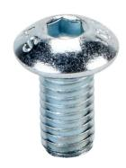
FATH button head socket cap screw, silver, M5-0.8 x 10mm, zinc plated steel, slot size 6/8/10. Package of 10. For use with all T-slotted rails. Manufacturer part number: 4ISO7380M0510M.
