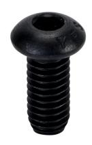
FATH button head socket cap screw, black, 5/16-18 UNC x 3/4in, zinc plated steel, slot size 8/10. Package of 10. For use with all 1.5in, 3in, 30mm, 40mm, 45mm, 60mm, 80mm and 90mm profile T-slotted rails. Manufacturer part number: 4ISO7380U,31-,75M.
