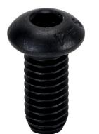
FATH button head socket cap screw, black, 5/16-18 UNC x 3/4in, zinc plated steel, slot size 8/10. Package of 10. For use with all 1.5in, 3in, 30mm, 40mm, 45mm, 60mm, 80mm and 90mm profile T-slotted rails. Manufacturer part number: 4ISO7380U,31-,75M.
