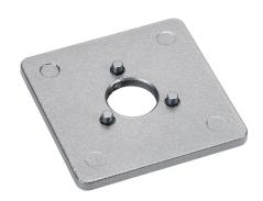
FATH fixed caster adapter plate, silver, 45 x 45mm, die-cast zinc, slot size 10. For use with 45 x 45mm profile T-slotted rails. Manufacturer part number: 098FA45N10.
