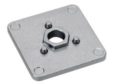
FATH fixed caster adapter plate, silver, 40 x 40mm, die-cast zinc, slot size 8. For use with 1.5 x 1.5in and 40 x 40mm profile T-slotted rails. Manufacturer part number: 098FA40N08.
