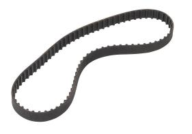
SureMotion timing belt, 1/5in XL pitch, 3/8in wide, 80 tooth, 16in pitch length (circumference), neoprene, fiberglass reinforced.
