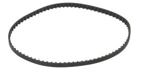
SureMotion timing belt, 1/5in XL pitch, 1/4in wide, 80 tooth, 16in pitch length (circumference), neoprene, fiberglass reinforced.
