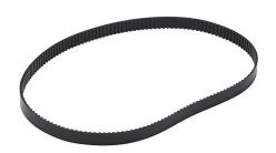
SureMotion timing belt, 0.08in MXL pitch, 1/4in wide, 160 tooth, 12.8in pitch length (circumference), polyurethane, polyester reinforced. Package of 3.
