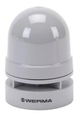
WERMA EvoSIGNAL Mini series audible signal horn, 95 dB at 1m, 4 kHz tone frequency, continuous/pulse tone(s), 12 VAC/VDC, modular mount, ABS/polycarbonate housing, gray, IP66. Requires mounting adapter.
