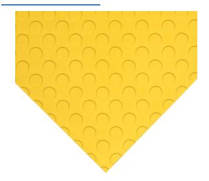
ASO Safety Solutions safety contact mat, 24 x 36in, straight edge, 24 VAC/VDC operating voltage, polyurethane contact surface, yellow, IP65, 4.7in/120mm cable length, (1) 3-pin male M8 connector and (1) 3-pin female M8 connector.
