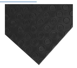
ASO Safety Solutions safety contact mat, 12 x 24in, straight edge, 24 VAC/VDC operating voltage, polyurethane contact surface, black, IP65, 4.7in/120mm cable length, (1) 3-pin male M8 connector and (1) 3-pin female M8 connector.
