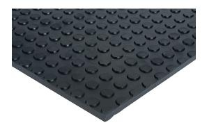
ASO Safety Solutions safety contact mat, 36 x 48in, straight edge, 24 VAC/VDC operating voltage, polyurethane contact surface, black, IP65, 4.7in/120mm cable length, (1) 3-pin male M8 connector and (1) 3-pin female M8 connector.
