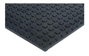
ASO Safety Solutions safety contact mat, 36 x 36in, straight edge, 24 VAC/VDC operating voltage, polyurethane contact surface, black, IP65, 4.7in/120mm cable length, (1) 3-pin male M8 connector and (1) 3-pin female M8 connector.
