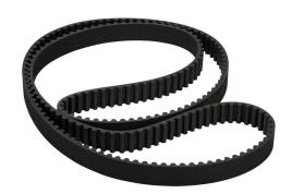
SureMotion timing belt, 8mm 8M pitch, 20mm wide, 200 tooth, 1600mm pitch length (circumference), neoprene, fiberglass reinforced.
