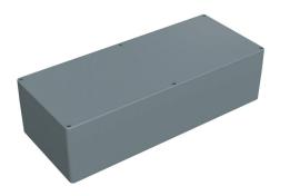
Hammond enclosure, NEMA 4/4X, 600 x 250 x 160mm (HxWxD), fiberglass reinforced polyester, RAL 7000 light gray, screw cover, purchase subpanel separately.
