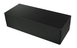
Hammond enclosure, NEMA 4/4X, 600 x 250 x 160mm (HxWxD), fiberglass reinforced polyester, black, screw cover, purchase subpanel separately.
