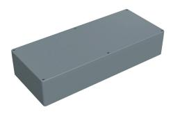
Hammond enclosure, NEMA 4/4X, 600 x 250 x 120mm (HxWxD), fiberglass reinforced polyester, RAL 7000 light gray, screw cover, purchase subpanel separately.
