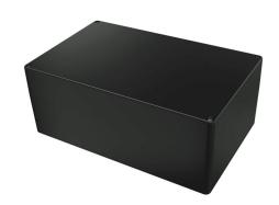
Hammond enclosure, NEMA 4/4X,  $400 \times 250 \times 160$ mm (HxWxD), fiberglass reinforced polyester, black, screw cover, purchase subpanel separately.
