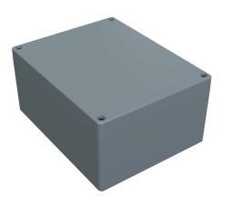
Hammond enclosure, NEMA 4/4X, 250 x 200 x 120mm (HxWxD), fiberglass reinforced polyester, RAL 7000 light gray, screw cover, purchase subpanel separately.
