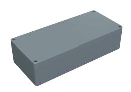
Hammond enclosure, NEMA 4/4X, 360 x 160 x 90mm (HxWxD), fiberglass reinforced polyester, RAL 7000 light gray, screw cover, purchase subpanel separately.
