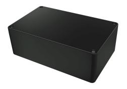
Hammond enclosure, NEMA 4/4X, 260 x 160 x 90mm (HxWxD), fiberglass reinforced polyester, black, screw cover, purchase subpanel separately.
