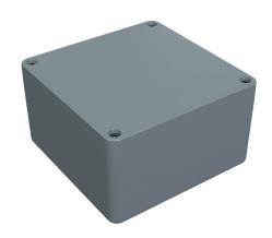
Hammond enclosure, NEMA 4/4X, 160 x 160 x 90mm (HxWxD), fiberglass reinforced polyester, RAL 7000 light gray, screw cover, purchase subpanel separately.
