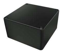
Hammond enclosure, NEMA 4/4X, 160 x 160 x 90mm (HxWxD), fiberglass reinforced polyester, black, screw cover, purchase subpanel separately.
